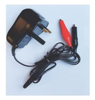
For charging 12v lead-acid batteries. Plugs directly into mains wall socket. Charge rate 720 mA approx. Features 'charge-complete' indicator and thermal fuse for safety. Instructions included.
