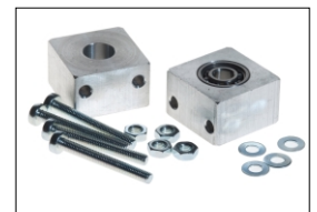
Bearing Blocks. 4mm I.D. (20 x 20 x 12.5mm) . 32g Part No: 918D10
