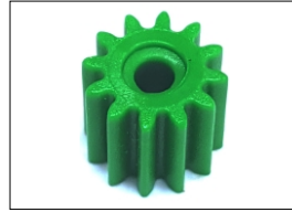
Pinions (Plastic) 12 tooth. 1.9mm I.D. 3g Part No: 917D2458
